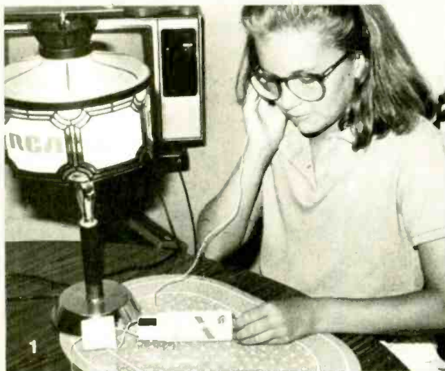
1 A pocket-size solar-cell radio was built inside a throw-away deodorant container. The chassis consisted of a cut-to-shape styrofoam piece on which to mount the solar cells and all the other radio components in the circuit.
