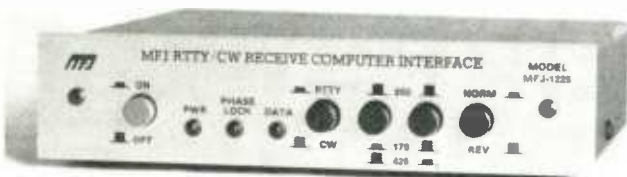
The model MFJ-1225 RTTY/CW Receiver-Computer Interface from MFJ Enterprises can be used to connect your computer to a ham-radio to decode Morse code and radioteletype signals. For more information circle No. 84 on Free Information Card.
