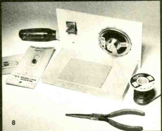
Two pieces of scrap material may be screwed together to form an inverted L chassis. Plastic or metal scrap may form the front panel, while compressed or white pine wood is used as the base. Few tools are needed to build this type chassis.
