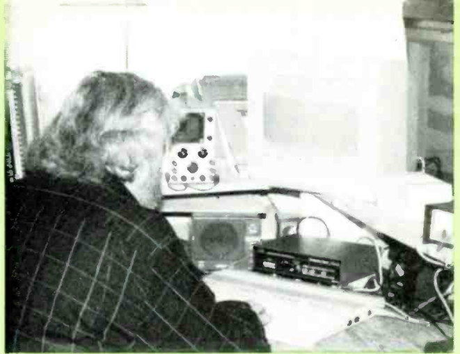
This new-age communications system—consisting of a Commodore C-128 computer, an AEA CP-1 interface with AEA software, and Kenwood TS-960S transceiver—can receive and transmit Morse code, AMTOR, ASCII, and RTTY.
