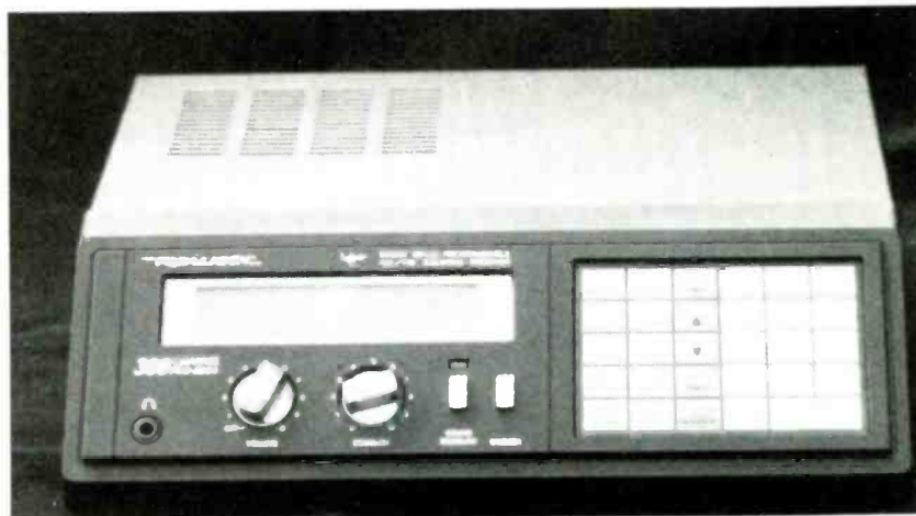
The Realistic PRO-2004 scanner features 300-channel coverage, 10 different search ranges, direct search (up/down) from any frequency shown on the LCD display, 10 scan banks, selectable mode (AM/NFM/WFM) for each channel; 5/12.5/50 kHz search steps, memory backup, bright/dim panel lights, and a feature that keeps the unit from stopping on inactive frequencies.
