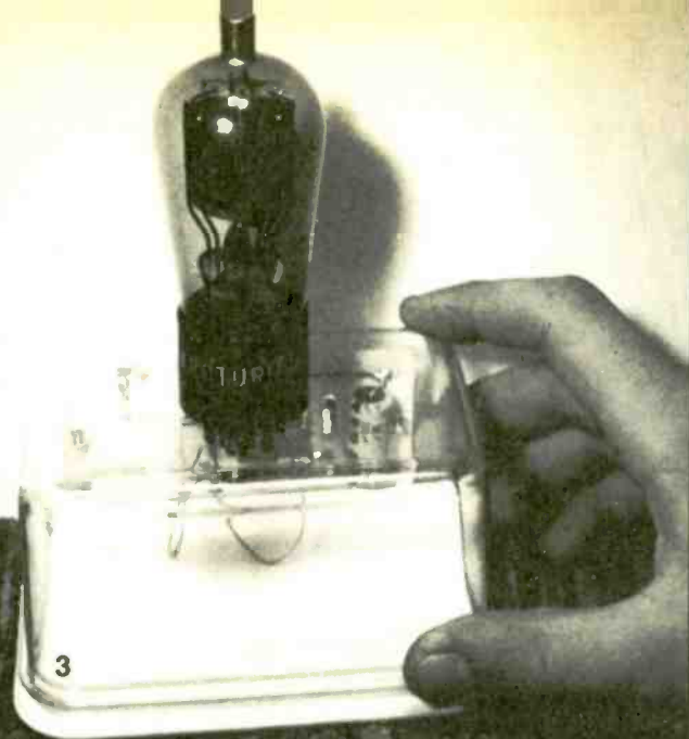
Clear plastic frozen-foods boxes may be used to house large electronics projects. Plastic boxes offer protection to small component parts and solar cells. Be careful not to crack the plastic sides when drilling small mounting holes.
